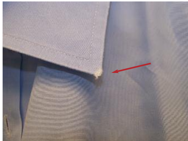
After normal, professional laundering of this shirt the fabric frayed and the interfacing poked through at the collar tips.
